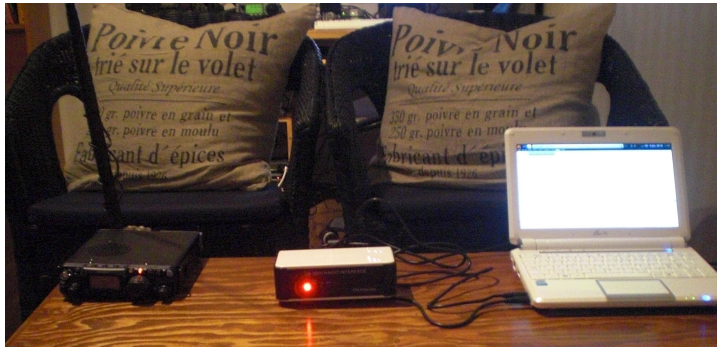
Illustration 1: SM0RWO portable setup, from left Yaesu FT-817ND, SB-2000 interface and EEE PC
